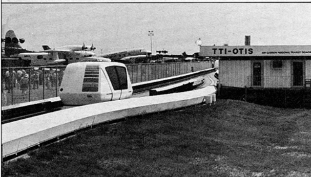
Dashaveyor-Bendix displayed the largest PRT vehicles for 31 riders and "crush" capacity for 44. For propulsion and guidance, the design utilizes rubber tires in a concrete channel while computers limit the speed to 20 mph.
