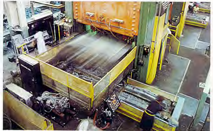
SMC strips for Chevrolet grille opening panels are automatically loaded into 2,000-ton press at General Motors Plant #6, Flint, Michigan.
