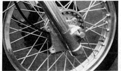
(Left) Lockheed caliper bites down on a cast-iron 11-inch disc; brake is powerful and predictable. Disc rusts on water contact. (Top Center) Control switches are unfortunate: too many bits-and-pieces and too hard to use. And the plumber's nightmare at the end of the brake reservoir should be sheathed in rubber. (Top Right) Instrument panel is handsome and well-angled, but the pilot lights are much too bright at night. (Center Below) SIs Grimeca rear brake works smoothly; mufflers are beautifully shaped. (Right Below) Right fork leg has boss for a brake caliper.
