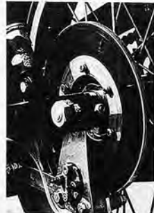
Rear brake: a fixed caliper, moving disc.
