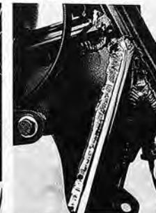
Steering head is heavily gusseted.
