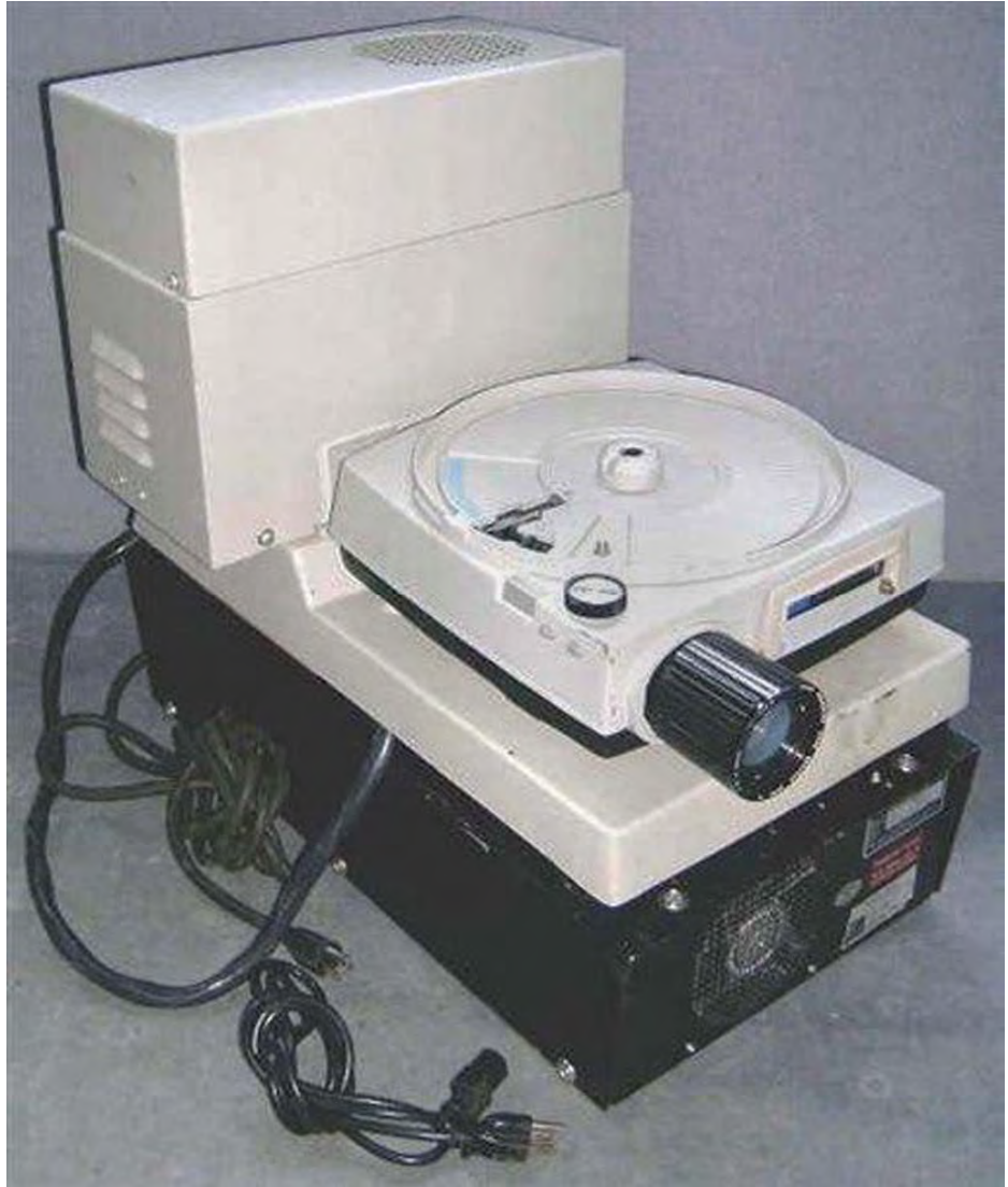
An ORC xenon-powered Kodak Carousel projector, 1986.
