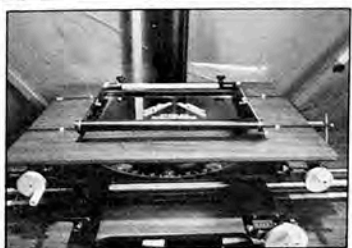
Close-up of Oxberry peg bars for producing multiple cell frames.
