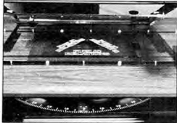
Heart of the system. Details of a Forox animation compound. Platen glass is placed on top of bottom-lit lithfilm negative. At front are handcranks for North, South, East and West movements, and peg bar movement.
