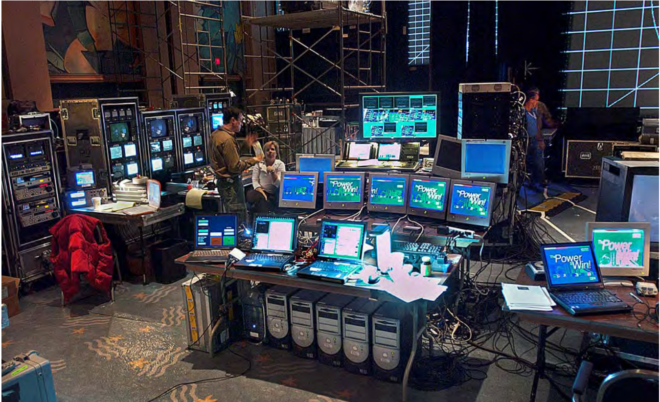
Back stage at the Orlando show. Laptop (right) controlled Watchout image serves (center). "Video Village" is seen at left.
