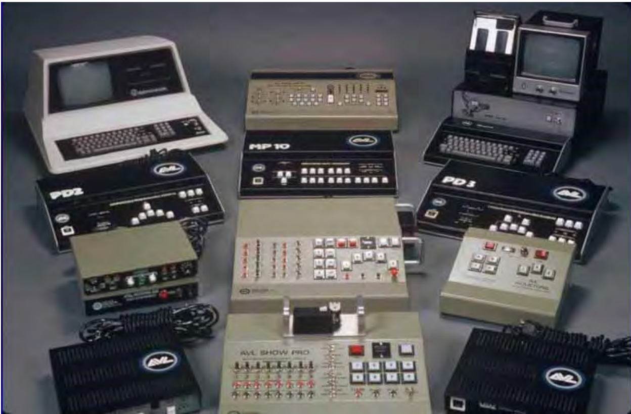
The family of slide-show control equipment manufactured by Audio Visual Laboratories between the mid-70s and mid-80s. First row (front): a Show Pro punch tape programmer flanked by PD-3 (left) and Dove (right) dissolvers. Second row: QD-3 dissolver (left), Show Pro II punch-tape programmer (center), Acuetone programmer (right). Third row: PD-2 programmer (left), MP-10 programmer (center), PD-3 programmer (right). Fourth row (back): Golden Eagle computer (left), Show Pro V digital programmer (center), Eagle computer (right).
